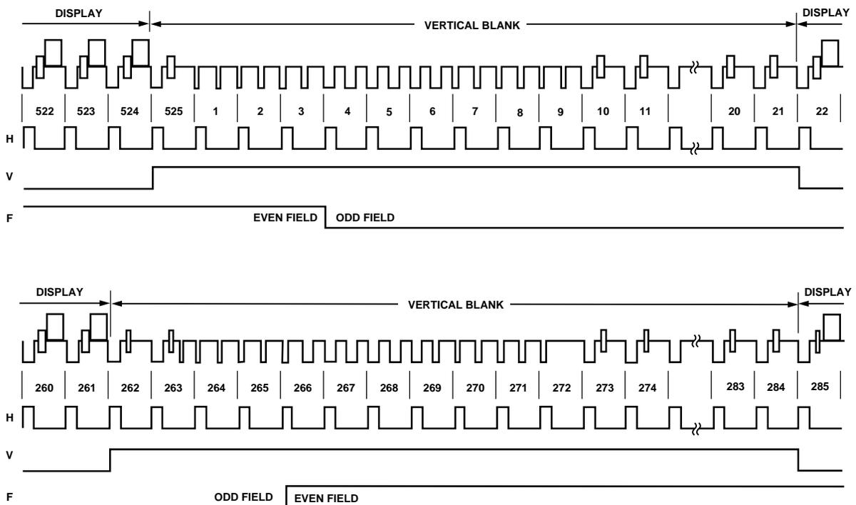
Figure 14. Timing Mode 0 (NTSC Master Mode)
