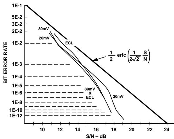
Figure 20. AD802-155 Bit Error Rate vs. Input Jitter
