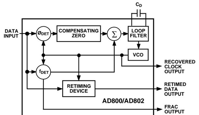
During the process of acquisition the frequency detector provides a Frequency Acquisition (FRAC) signal which indicates that the device has not yet locked onto the input data. This signal is a series of pulses which occur at the points of cycle slip between the input data and the synthesized clock signal. Once the circuit has acquired frequency lock no pulses occur at the FRAC output.
