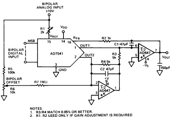
Figure 23. AD647 Used as DAC Output Amplifier
