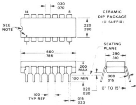
NOTE LEAD NO 1 IDENTIFIED BY COLOR DOT OR NOTCH MECHANICAL INDEX POINT OR NOTCH IN PIN
