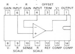
controlled load applications. A separate output reference terminal is also provided so that the output can be biased independently of the gain setting.
