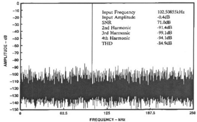
Figure 20. Full-Scale Power Spectral Density after Power-up at  $T_{CASE} = +25^{\circ}C$  Without Calibration,  $\pm 5$  V Range, 16384-Point FFT, 500 kHz Sample Rate. Compare with Figure 4.
