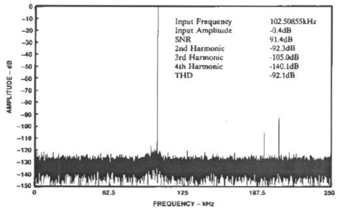
Figure 22. Same as Figure 21 Following Recalibration at  $T_{CASE} = +125^{\circ}C$
