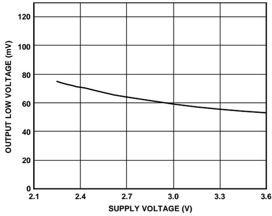
Figure 9. Output Low Voltage vs. Supply Voltage
