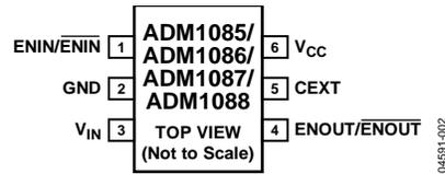
Figure 2. Pin Configuration
