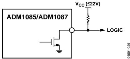
Figure 21. Open-Drain Output Stage
