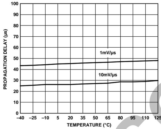
Figure 10.  $V_{CC}$  Falling Propagation Delay vs. Temperature
