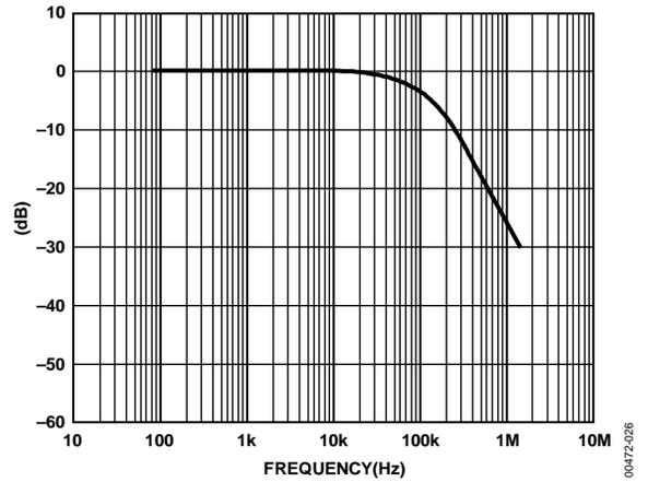
Figure 22. Multiplying Bandwidth (Small Signal Frequency Response)
