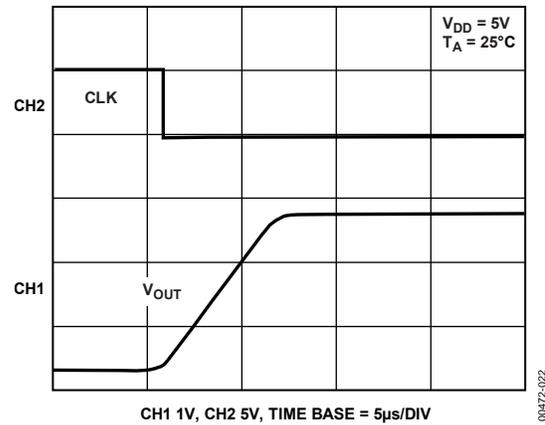
Figure 18. Half-Scale Settling (1/4 to 3/4 Scale Code Change)
