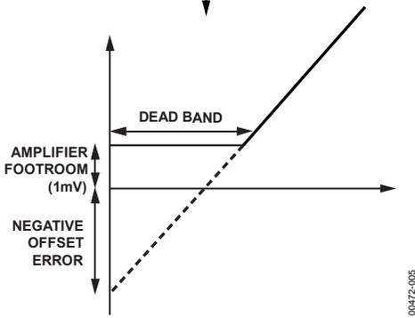
Figure 3. Transfer Function with Positive Offset
