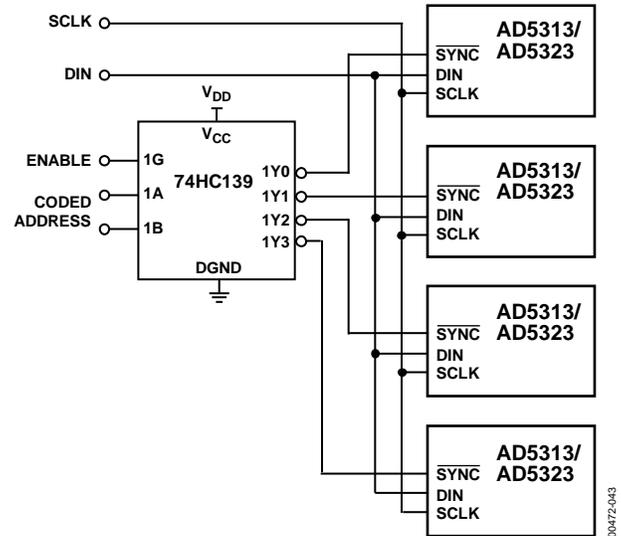
Figure 38. Decoding Multiple AD5313/AD5323 Devices in a System
