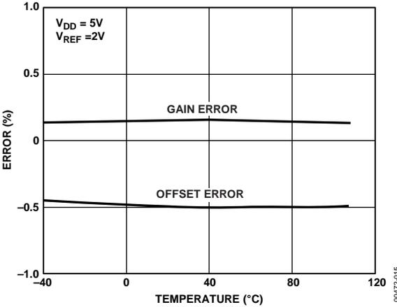
Figure 11. Offset Error and Gain Error vs. Temperature
