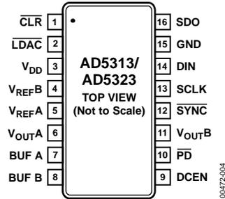
Figure 6. Pin Configuration
