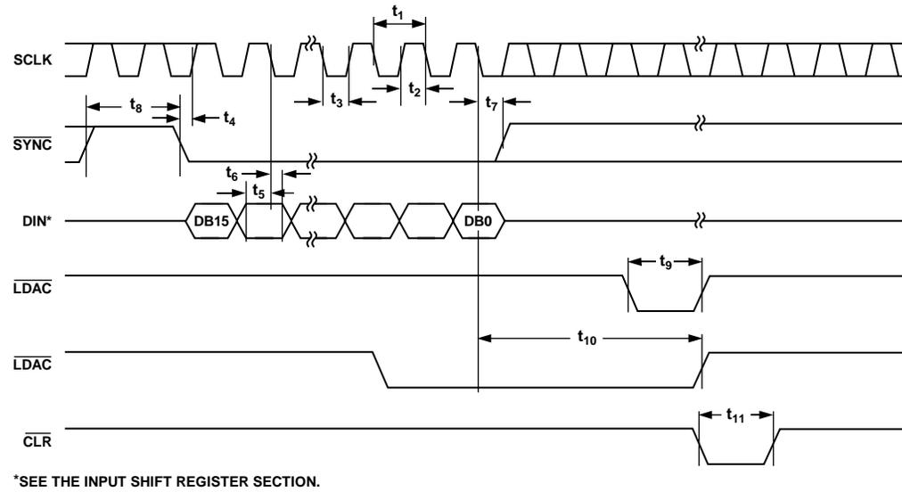
Figure 5. Serial Interface Timing Diagram
