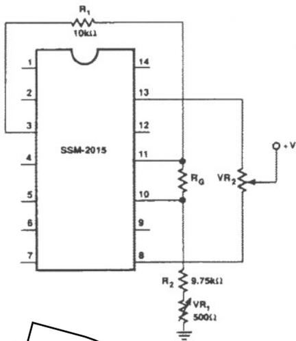
FIGURE 4: Trimming the SSM-2015
