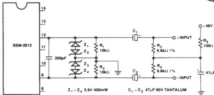
FIGURE 5: SSM-2015 with Phantom Power
