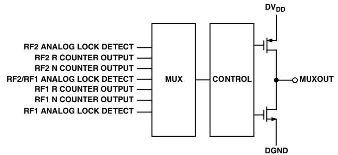
Figure 6. MUXOUT Circuit
