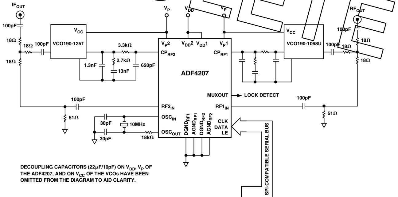
Figure 7. GSM Handset Receiver Local Oscillator Using the ADF4207
