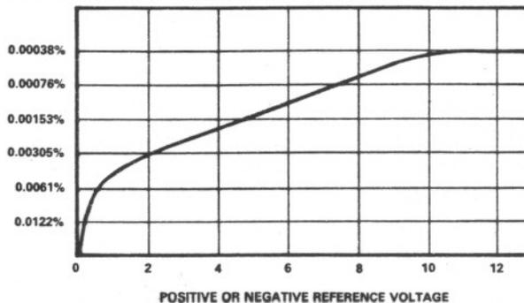
Figure 5. Typical Differential Linearity vs. External Reference Voltage
